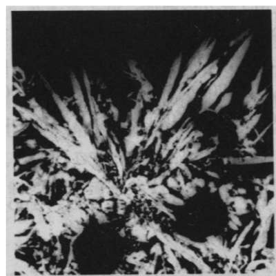
Fig. 2 Optical polarizing micrograph of polyester CP4, focal-conic texture, obtained at 165 ^{\circ}\text{C} ( \times 320 )
